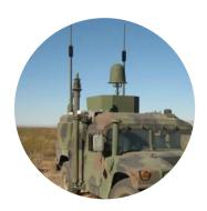
The **SAS-200 Series** are dual band omni antennas with a discone low-band construction and either a conical monopole for the 3 GHz configuration or vertical biconical for the 6GHz and 18GHz configurations. These antennas are available with a diplexed output option or a high and low band output.
